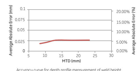
Accuracy curve for depth profile measurement of weld height.
